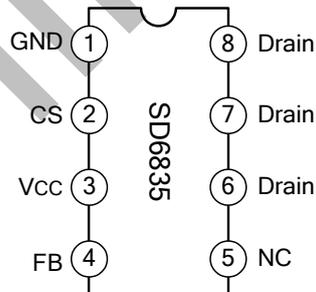
**Note:** it is recommended to connect pin 5 to pin Drain for better heat dissipation.
