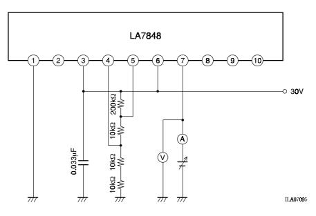
In the circuit in figure 3, read the value shown by the voltage meter (V) when the current meter (A) reads 20mA.
