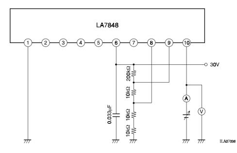
In the circuit in figure 6, read the value shown by the voltage meter (V) when the current meter (A) reads 500mA.
