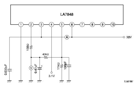
In the circuit in figure 5, read the value shown by the current meter (A). In the circuit in figure 5, read the value shown by the voltage meter (V).
