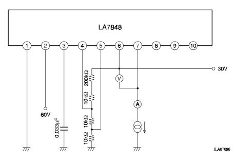
In the circuit in figure 4 with the output from pin 7 absorbed by an electronic load, read the value shown by the voltage meter (V) when the current meter (A) reads 1.1A.
